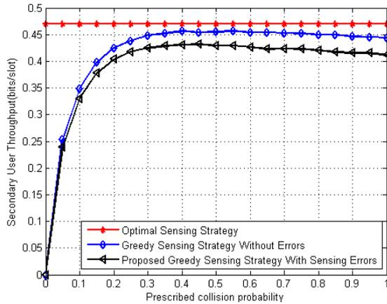
**Fig. 8** Performance of the proposed scheme in presence of sensing errors for equal bandwidth and equal transition probabilities.
