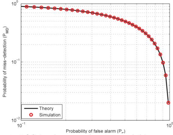
**Fig. 5** ROC (receiver operating characteristic) curves for energy detector.
