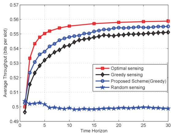
**Fig. 10** Performance of the proposed scheme using greedy sensing algorithm: 3 independent channels with equal bandwidth and equal transition probability.
