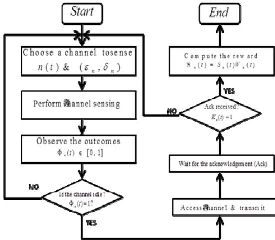
**Fig. 4** A simplified one time slot transmission protocol.
