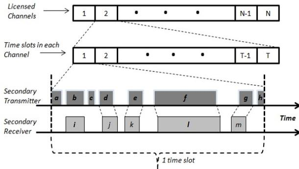
**Fig. 3** A sequence of operations in one time slot for proposed MAC scheme.
