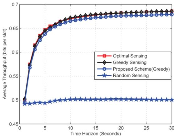
**Fig. 9** Performance of the proposed scheme under greedy sensing algorithm: 3 independent channels with equal bandwidth and equal transition probabilities.
