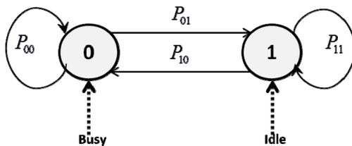
Fig. 1 Two states discrete Markov model for a single channel.
